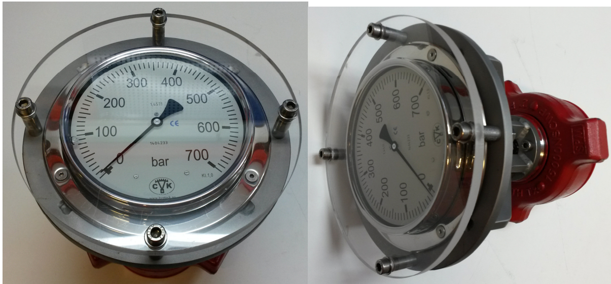
Figure 9 & 10 Pressure Gauge unit with 0-700Bar scale
